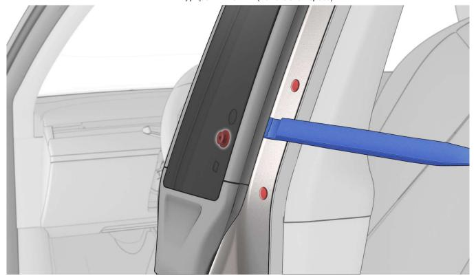
4. Release the trim clip that attaches the upper portion of the B-pillar applique to the B-pillar.
