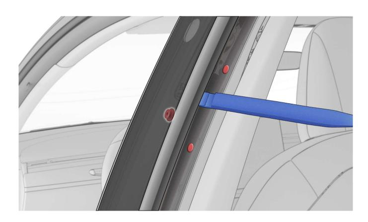
5. Slide the B-pillar applique down slightly to release the assembly from the body, and then disconnect the camera connectors from the B-pillar applique.
