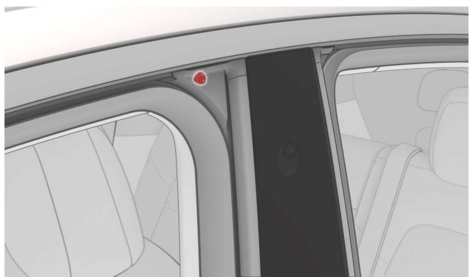
**5.** Gently press the double sided tape that attaches the lower portion of the B-pillar applique sea to the vehicle.
