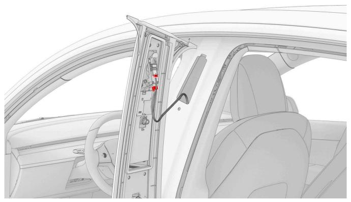
**3.** Position the B-pillar applique onto the vehicle, and then engage the clips that attach the B-pill applique to the vehicle.
