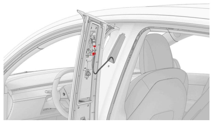
6. Release the clip that attaches the B-pillar applique seal to the vehicle, and then remove the applique from the vehicle.
