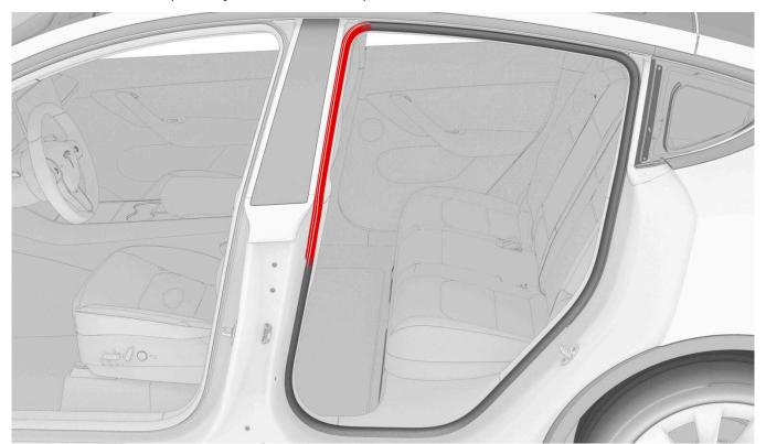
3. Release the trim clip that attaches the lower B-pillar applique to the B-pillar.
